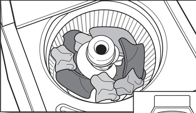
Load garments in loose heaps evenly around basket wall. For best results, do not pack the load tightly. Maximum load size (as tested) is 7.7 kg. Do not wrap large items such as sheets around the agitator; load them in loose piles around the sides of the basket. Try mixing different sized items to reduce tangling.
