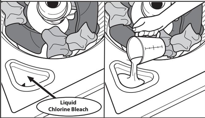
Do not overfill, dilute, or use more than 250 mL (1 cup). Do not use color-safe bleach or Oxi products in the same cycle with liquid chlorine bleach.
